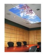
Sky Factory SkyTile Elevators (patent pending) further contribute to the illusion. "Elevators" are aluminum extrusions that transform the standard ceiling grid into a structure that, because of perceptual habits, looks to the mind like the extrusions used to support a real skylight. Again, by modifying the cognitive process, the mind is tricked into "knowing" that what is actually on all sides of such a structural grid must be "beyond" – like a real sky.
